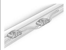
If the level of the shoulder is only slightly below the pavement, recovery should be fairly easy. Ease off the accelerator and then, if there is nothing in the way, steer so that the vehicle straddles the edge of the pavement.
